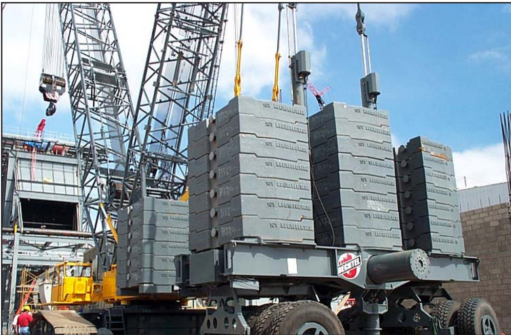
Figure 3.6-4B Super Lift Configuration of a Crawler Crane
